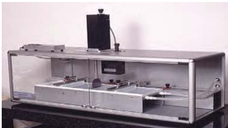
Figure 9.2. KSV 3000 model Langmuir-Blodgett device.
