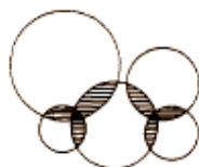
Figure 10.19. Schematic presentation of the overlap of hemispherical centers growing on a monolayer (progressive nucleation).
