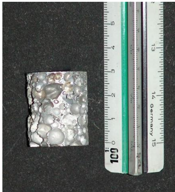
Figure 6.6. Cylindrical foam sample for effective thermal conductivity test.
