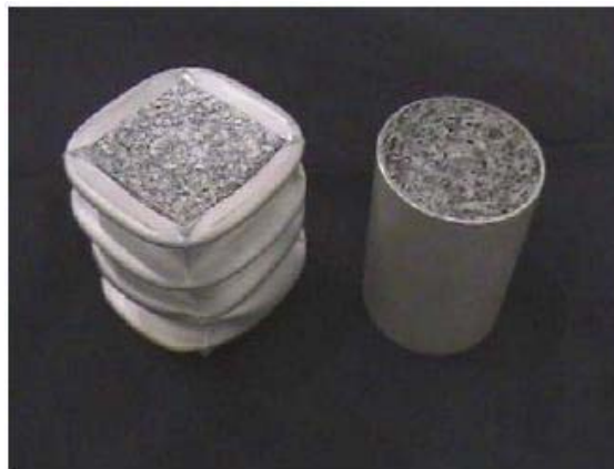
Figure 3.3. Examples of foam filled tubes. (Source: Banhart 2003)
