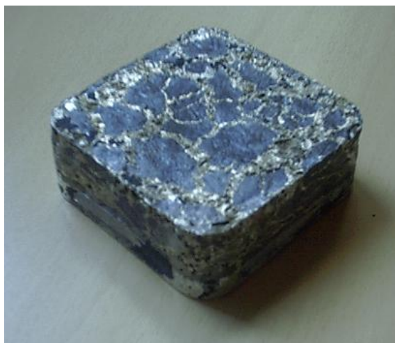
Figure 6.4. Al foam sample after cooling process.
