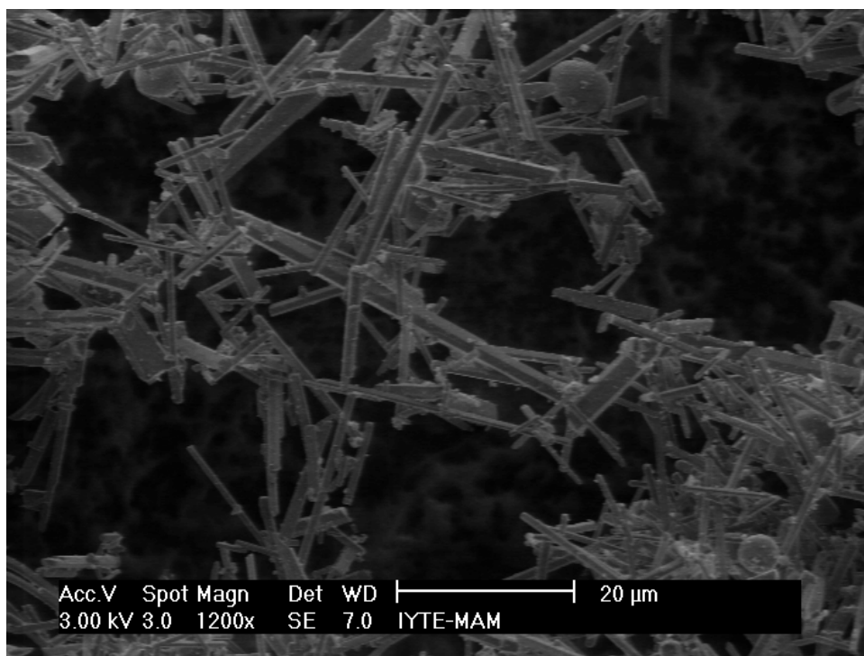
Figure 5.23. SEM image of wet mixed commercial HA powder KW7 whiskers synthesized at 1150°C where K_2SO_4/HA ratio during preparation was 3/1.
