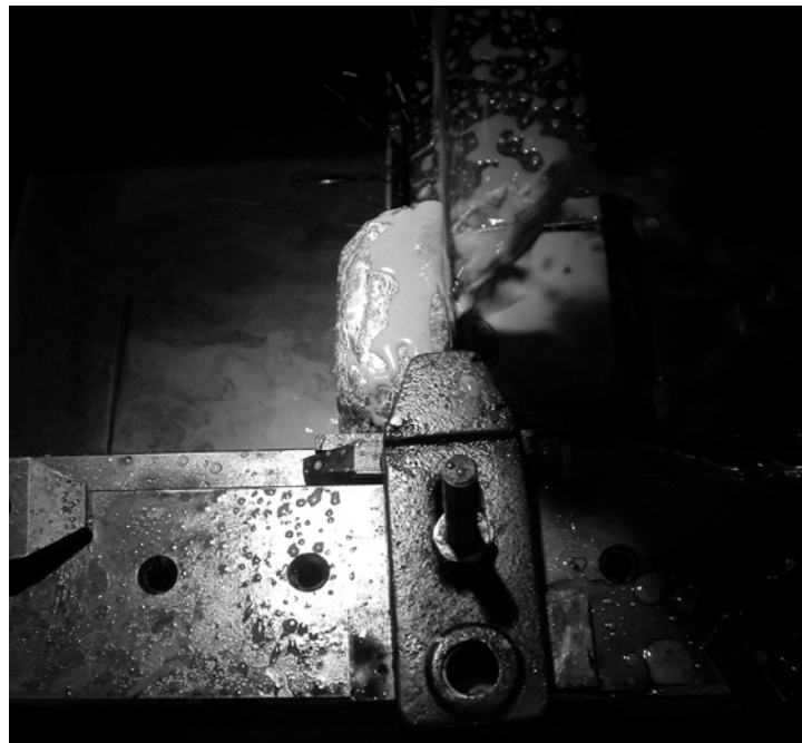
Figure 4.9. View of machining foam fillers using electrical discharge machine.
