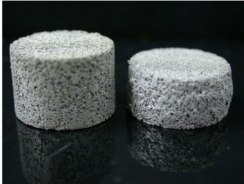
Figure 5.29. Undeformed and deformed images of the foam: P= 500 MPa, T=1300 °C, t=6 h.
