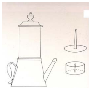
Figure 3.22. Section drawing of the de Belloy pot of about 1800 with filter basket and rammer (Source: Bramah E. and Bramah J. 1995)
