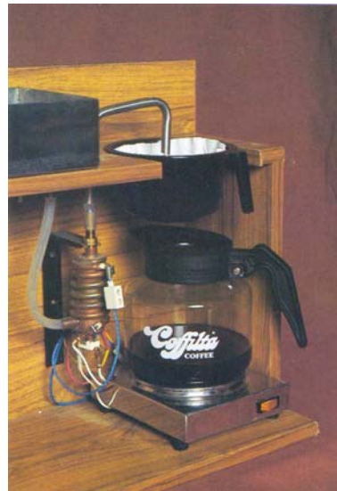
Figure 3.86. Coffilta coffee machine illustrating the simple mechanics behind the modern automatic filter machine fitted with a flow boiler (Source: Bramah E. and Bramah J. 1995)
