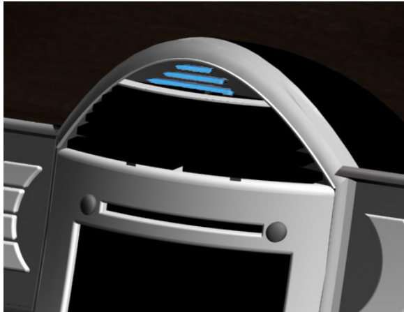
Figure 6.3. The park sensor's led is top of the right instrument panel.
