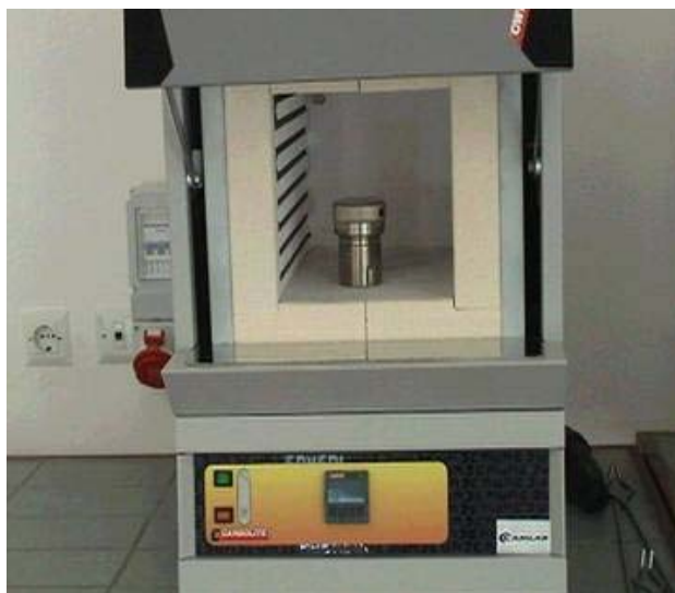
Figure 2.3. Carbolite CWF 1100 oven
