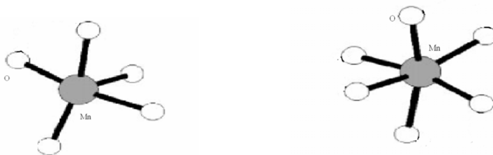
Figure 3.4. Ball and stick representation of \text{MnO}_5 (a) trigonal bipyramid and \text{MnO}_6 (b) octahedra.
