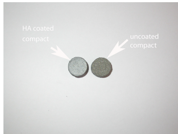
Figure 6.30. Sol-derived HA powder coated and uncoated Ti6Al4V sintered power compacts
