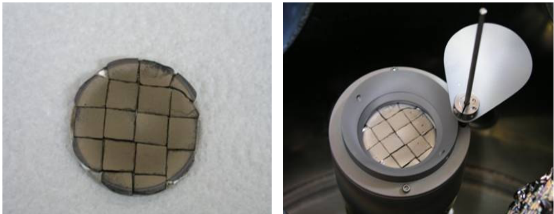
Figure 3.4. MgB 2 /Mg target top view and located in sputtering head.
