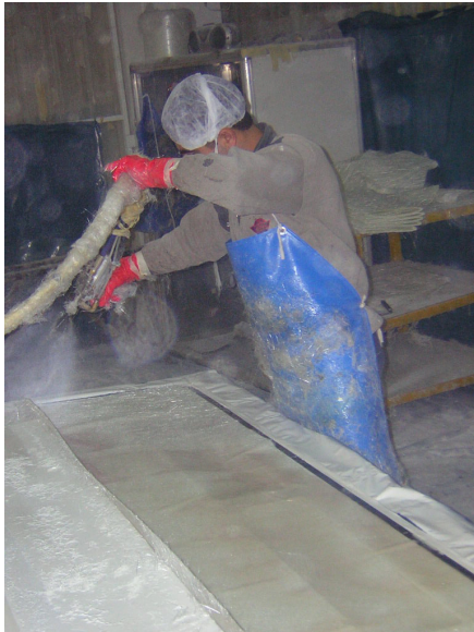
Figure 5.21. Polijel Applications on PRO X Cover Mould by Spray Gun.
