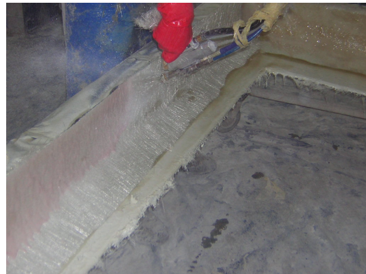
Figure 5.21. Polijel Applications on PRO X Cover Mould by Spray Gun.
