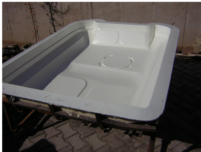
Figure 5.25. Drying Phase of PRO X Mould under the Sun
