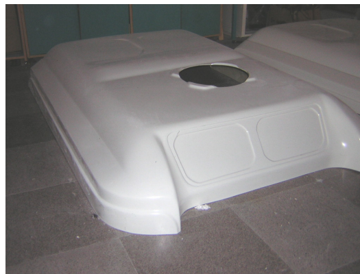
Figure 5.23. Polyester PRO X Cover taken out of Mould
