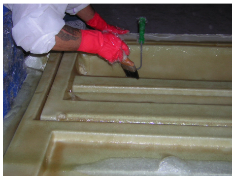
Figure 5.22. Polijel Application on PRO X Cover Mould by Hand lay-up.
