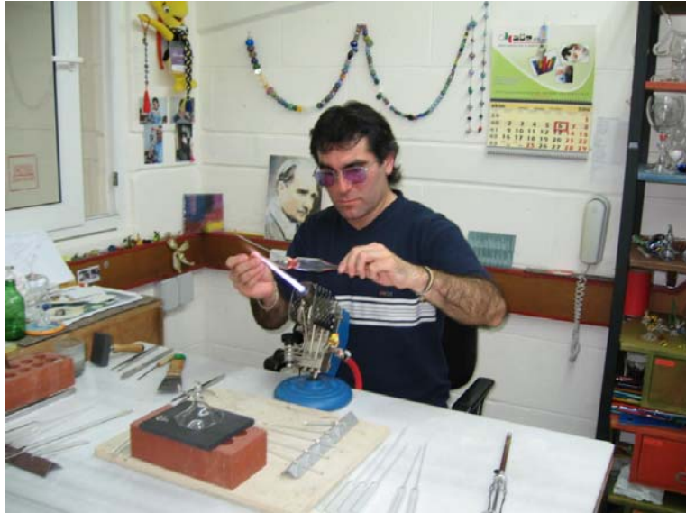
Figure 3.18. Shaping by heating on table.
