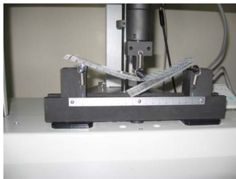
Figure 6.9. After the applied bending test, the reinforced PMMA plate breaks down
