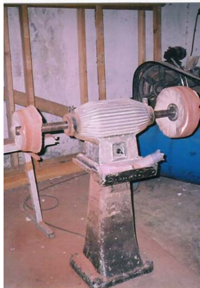
Figure 2.15. The rough surfaces are straightened by the emery machine
