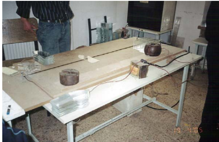
Figure 2.13. PMMA, which has been turned into panels, is shapened by cutting.
