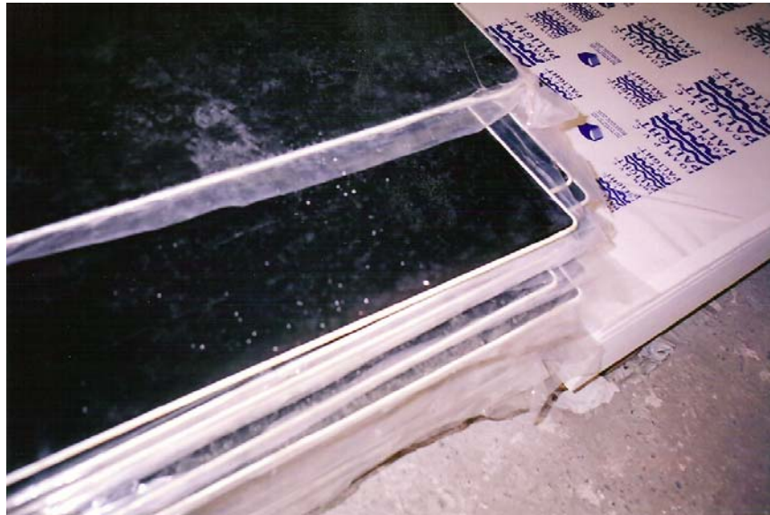
Figure 2.8. The wicks stay around the PMMA panels which are taken out from the mould.
