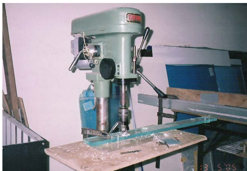
Figure 2.14. The holes are opened by means of the drill.
