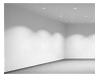
Figure 2.3. Direct, aimed lighting
