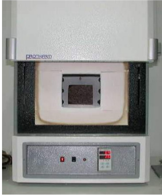
Figure 4.2.1. Protherm PLF 160/5- High Temperature Furnace (Max. Temp.=1600°C).
