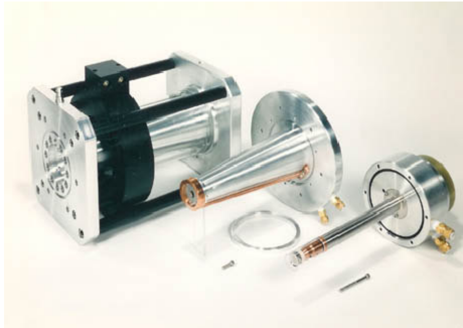
Figure 3.7. MEVVA ion source disassembled (Source: Web_2, 2006)
