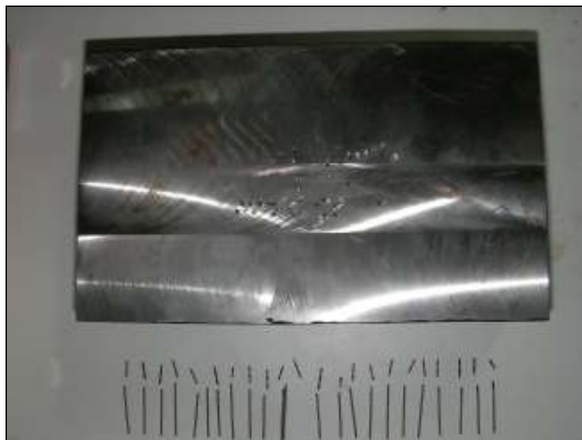
Figure 4.7. The broken drill bits
