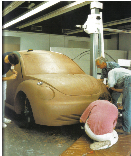
Figure 3.67. Clay modeling and data measuring
