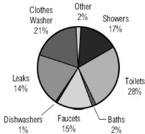
Figure 4.7. Typical water use (per person) in an American single family home. (Source: AWWA Residential End Use Study, 1999)
