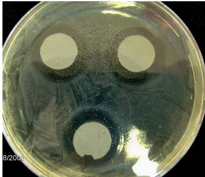
Figure 22. Antimicrobial activity of porous surfaces of cellulose acetate films on E. coli . The films were prepared with CA/acetone/water/lysozyme/EDTA weight percentages of 5/80/12.3/1.5/1.2.
