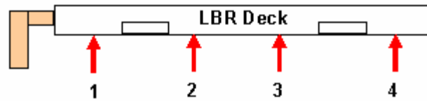
Figure 6.2. Thermocouple locations on the fin deck (front side).
