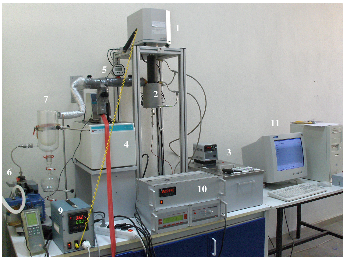
Figure 7.3. Digital photograph of experimental set-up in laboratory. 1, balance; 2, sorption cell; 3, circulating water bath; 4, water bath; 5, pressure transducer; 6, vacuum pump; 7, cold trap; 8, heating tape; 9, temperature controller; 10, control unit; 11, computer
