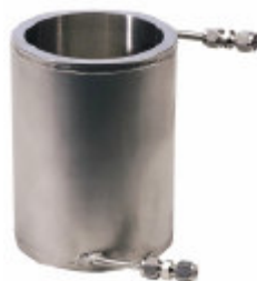
Figure 7.4. Double walled jacket for thermostating measuring cell with a circulating fluid (Source: WEB_2 2007)
