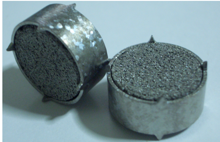
Figure 5.27. Third Prototype with supporting pins and jackets.
