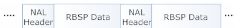
Figure 3.4. Sequence of NAL units each combined with NAL Header and RBSP Data
