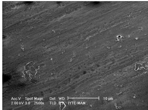
Figure 4.58. SEM image of IPS Empress 2 veneer in 0.25M CaCl 2
