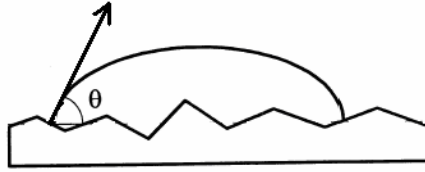
Figure 4.63. Apparent Contact Angle for an Asymmetric Rough Surface
