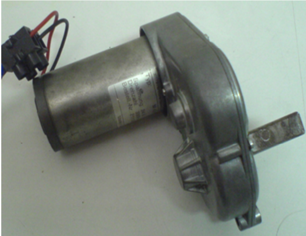
Figure 2.10. Actuator of the wearable exoskeleton robot (DC electric Motor).
