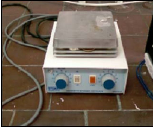
Figure 4.4. Picture of hot plate used for soft and hard baking
