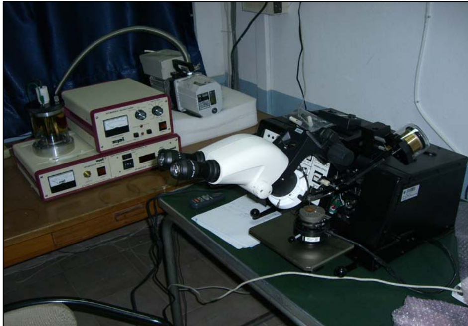
Figure 4.8. Wire bonder used for contacts
