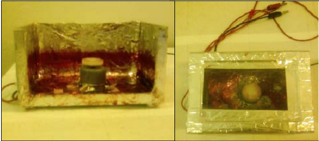
Figure 4.3 Pictures of home made spinner used for photoresist coating
