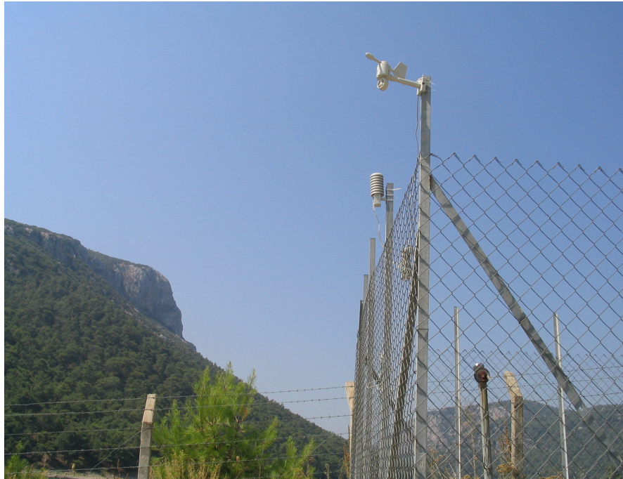
Figure 6.7. Meteorological station set up at Southwest location of the lake to record the meteorological data required as an input to the numerical model
