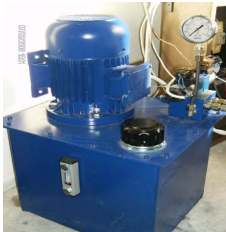
Figure 4.5. Hydraulic Power Unit
