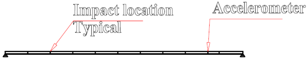
Figure 4.4. Sensor and Impact Locations of Test Structure
