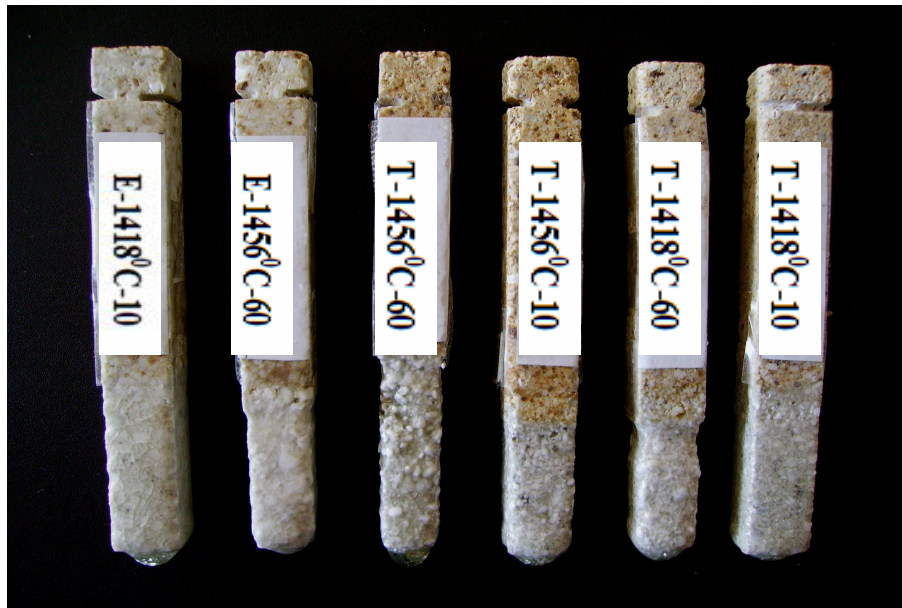
Figure 5.16. A photograph of the corroded refractory bricks after dynamic corrosion tests. (E-1418-10: E refractory specimen was tested at 1418 C during 10 minutes)
