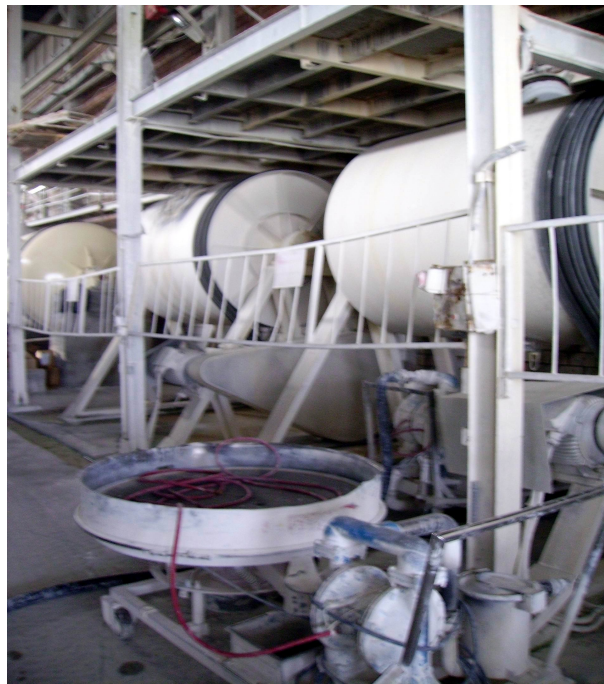
Figure 2.12. The grinding process (Grinding the frit in ball mill, Graniser A.Ş.)
