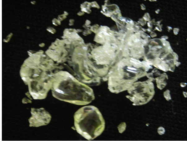
Figure 2.8. Frit (transparent frit granules)
