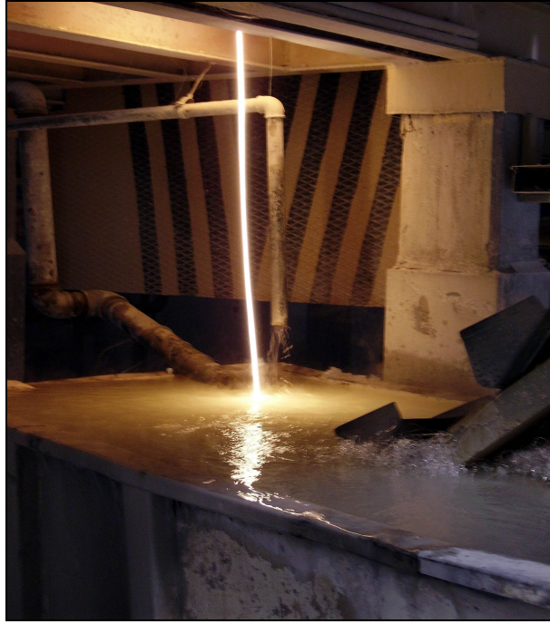
Figure 2.11. The quenching process (Discharging the frit into water, EgeSeramik A.Ş.)
