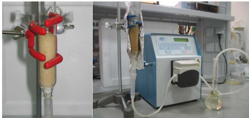
Figure 4.3. Color change in silk fibroin after adsorption
