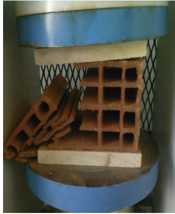
Figure 3.4. Test specimen of set1 after loading
