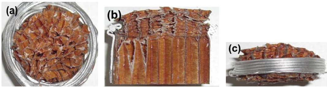
Figure 4.15. Deformed 3.2 mm cell size honeycomb filled tubes (a) top view, (b) cross-section and (c) side view
