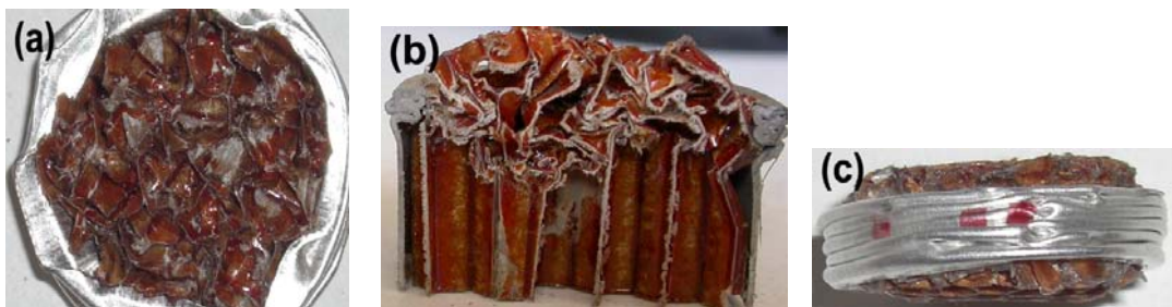
Figure 4.16. Deformed 4.8 mm cell size honeycomb filled tubes (a) top view, (b) cross-section and (c) side view
