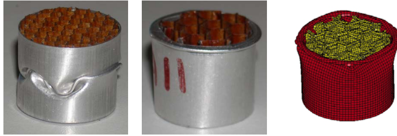
Figure 5.13. Deformed filled tubes, (a) trigger at the mid-section, (b) trigger from the end of the tube and (c) numerical deformation triggering from the tube end
