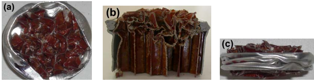
Figure 4.17. Deformed 6.4 mm cell size honeycomb filled tubes (a) top view (b) cross-section and (c) side view
