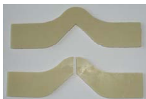
Figure 3.7. Tear test specimen before and after the tear test
