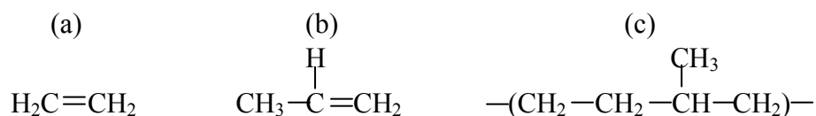
Figure 2.6. Structure of (a)ethylene, (b)propylene and (c)copolymer of ethylene and propylene (Source: Dick and Anicelli, 2001)
