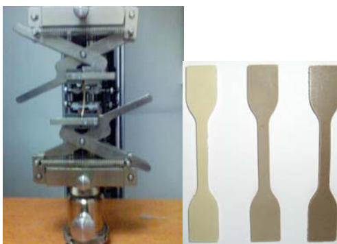
Figure 3.6. Photo of tensile test and tensile test specimen
