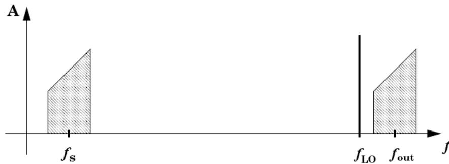
Figure 3.4. Frequency representation of upconversion
