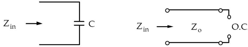
Figure 4.34. Input impedance of an open-circuit transmission line section and a capacitive lumped-element
