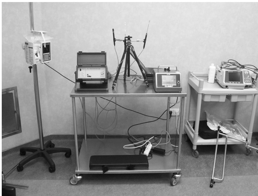
Figure 9.11. Data logger, transducers and particle counter set-up in the operating room environment
