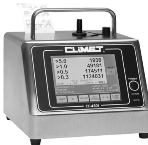
Figure 9.3. Climet CI-450t particle counter (Source: Climet Instruments Company 2007)
