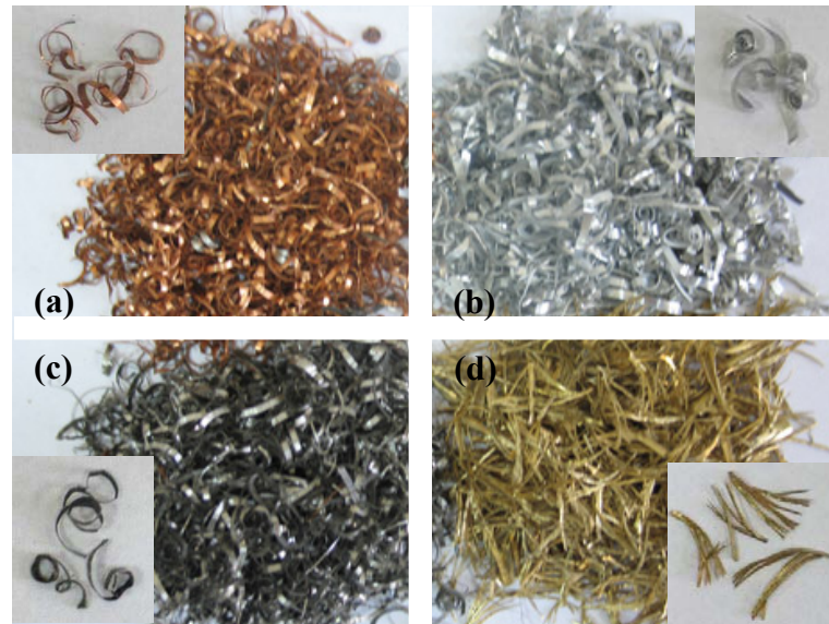
Figure 4.1. A photograph of used metal pieces a) Copper b) Aluminum c) Stainless steel d) Brass
