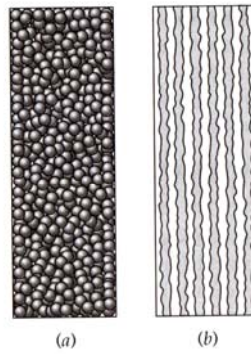
Figure 7.1. a) Porous packed bed having cylindrical shape b) tube bundle model (Source: Bird, et al. 2002)
