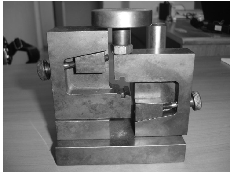
Figure 4.10. V-Notch Test Apparatus
