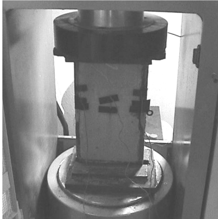
Figure 6.3. GFRP Strengthened Steel Plate Test Set-up
