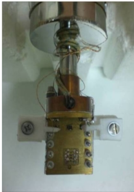
Figure 3.8. The cold finger with a chip mounted and contacts affixed.
