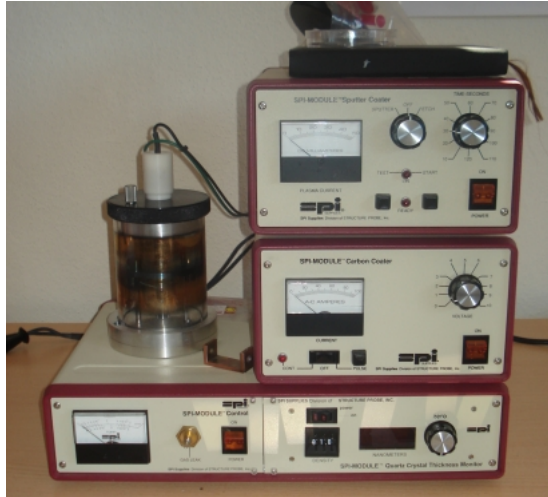
Figure 3.6. The SPI™ sputter coater used for contact metallization.
