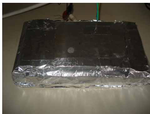
Figure 3.4. The homemade hot plate used in patterning.
