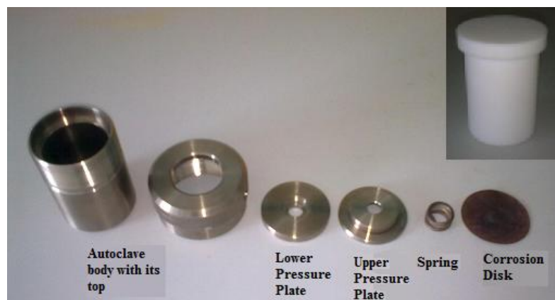
Figure 2.1. Schematic representation of an autoclave with its parts. (Inset shows the Teflon liner)
