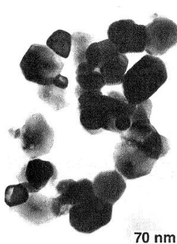
Figure 1.5. TEM image of powders prepared with Ce-HMT calcined at 450°C. (Source: Chen and Chen 1993)
