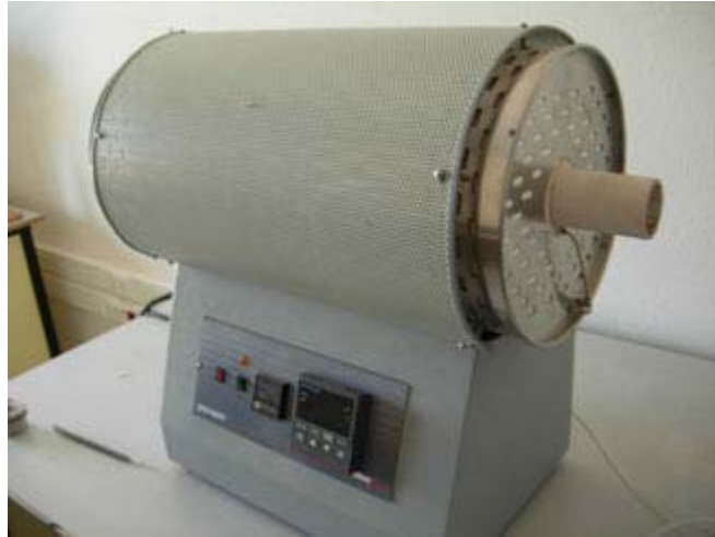
Figure 3.1. Tube furnace used for dry oxidation.
