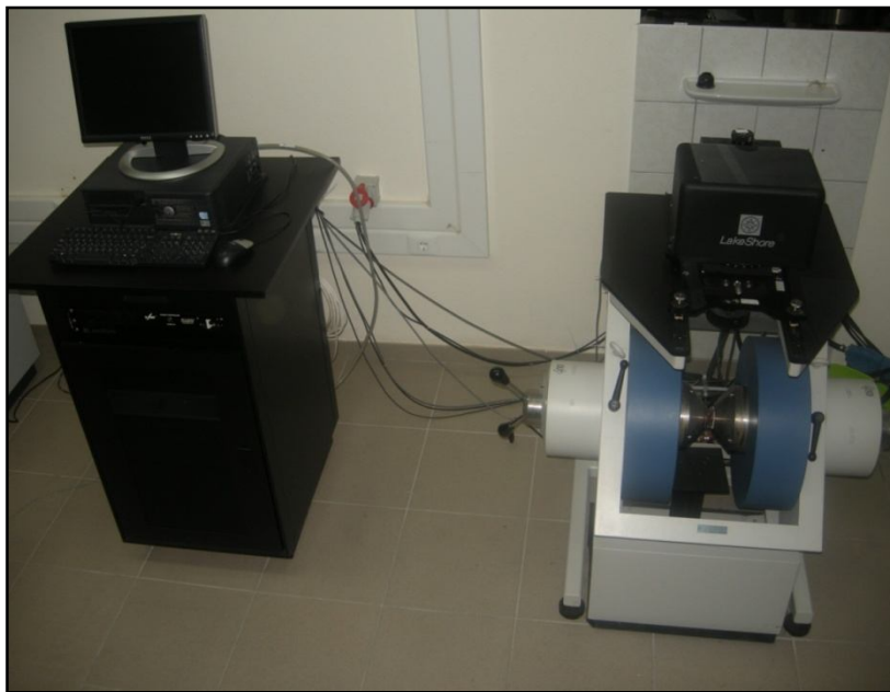
Figure 3.11. Lakeshore 7400 Vibrating Sample Magnetometer (VSM).
