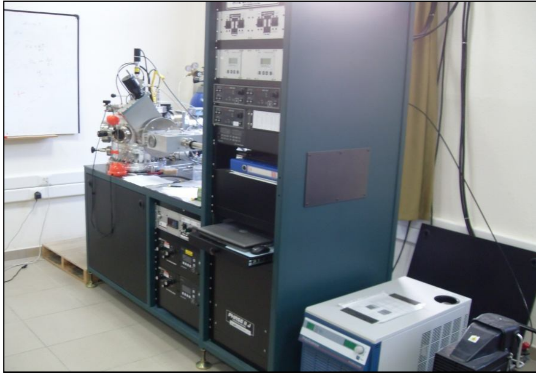
Figure 3.2. ATC ORION 5 UHV Magnetron Sputtering System.
