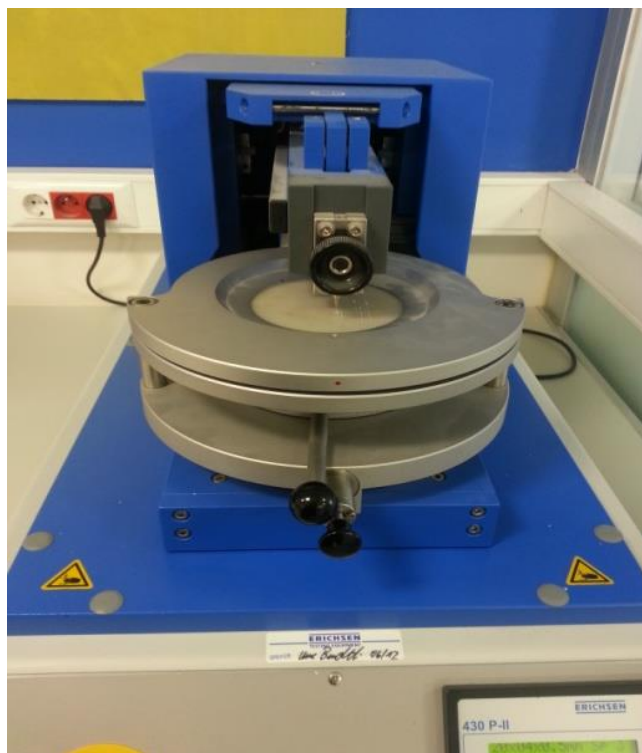
Figure 3.5 : Erichsen scratch tester.
