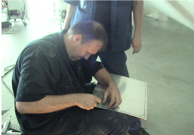
Figure 6.5 Preparing an External Doubler
