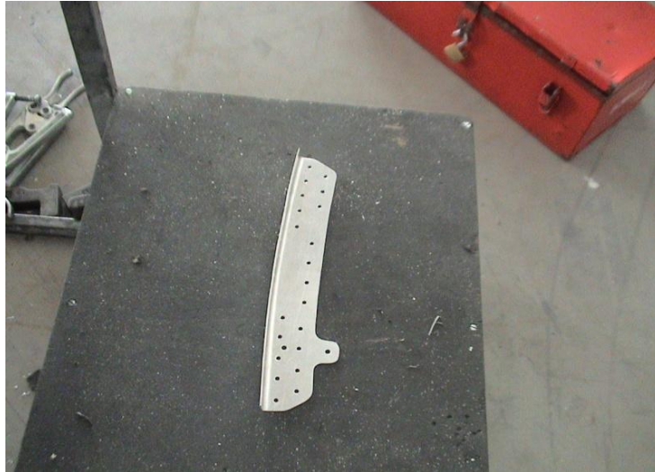
Figure 6.3 Preparing Filler for Fuselage Skin Repair
