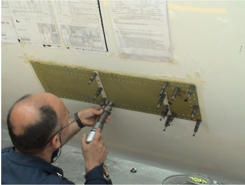
Figure 6.21 Fuselage Repair (Installation of the Rivets)
