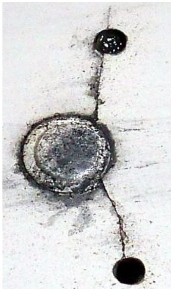
Figure 1.9 Crack Propagation on the Fuselage [15]
