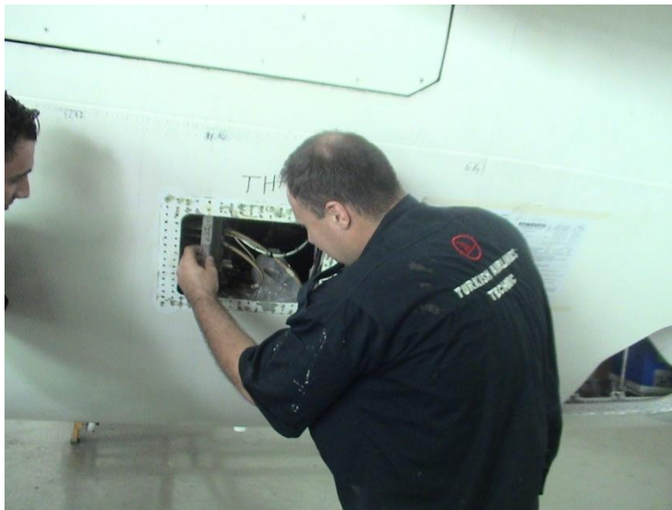
Figure 6.6 Checking of the Repair Area
