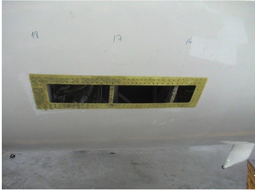
Figure 6.19 Fuselage Repair (Cut-out)
