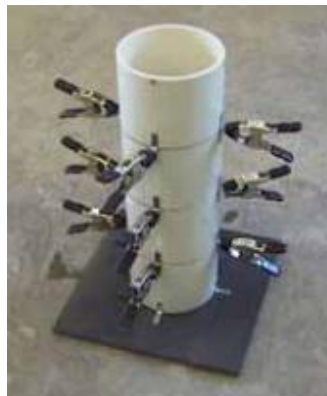
Figure 2.6. The column segregation test [13]
