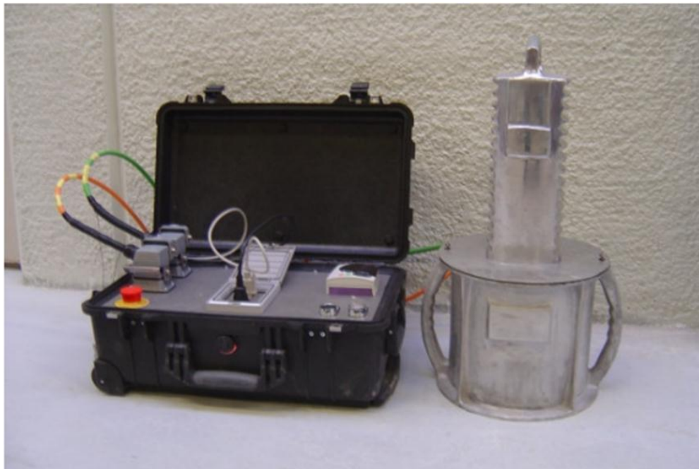
Figure 3.4. Contec 4SCC rheometer
