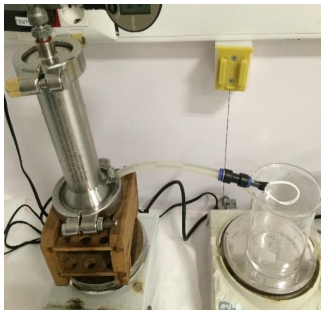
Figure 3.5 : Modified Sterlitech for HF membranes.
