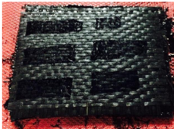
Figure 4.7 : A view of patterned nano-stitch on customize prepreg ply.
