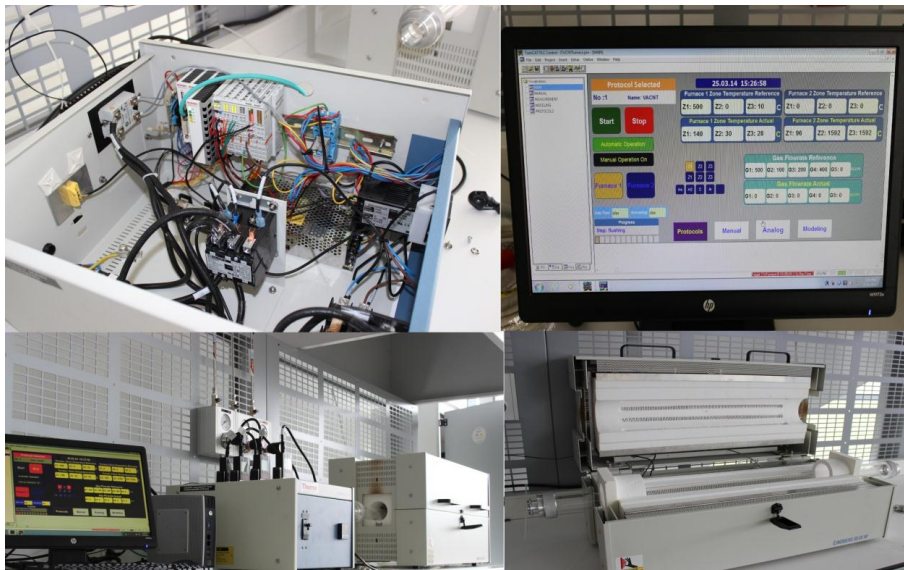
Figure 3.2 : Picture of customized CVD system.
