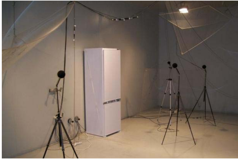
Figure 5.2 Reverberation room to test the sound power level
