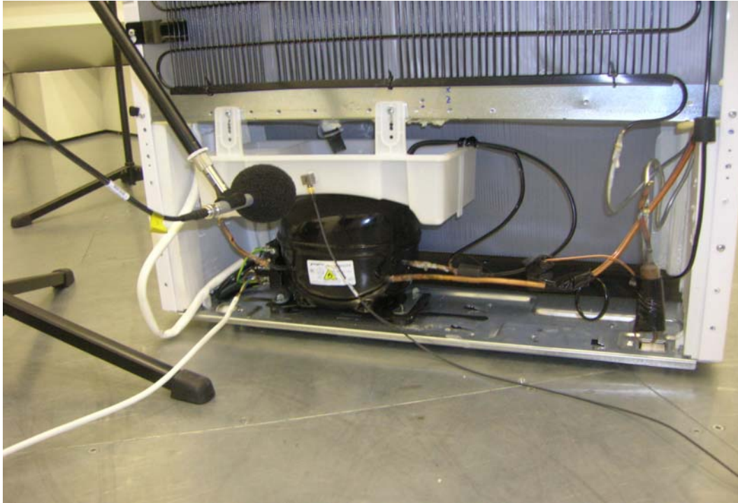
Figure 4.2. Cabinet base plate cross-spectrum test set-up
