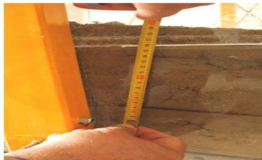
Figure 5.9. Infiltration (wetting band) Depth Measurement after the Experiment
