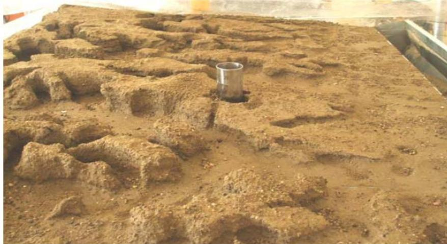
Figure 5.10. Shelby Tube used to obtain Undisturbed Soil Samples after Rainfall.
