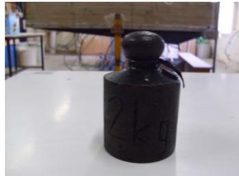
Figure 5.15. 1-D Experiments - Soil Compaction via 2 kg Weight/10cm Soil Layer
