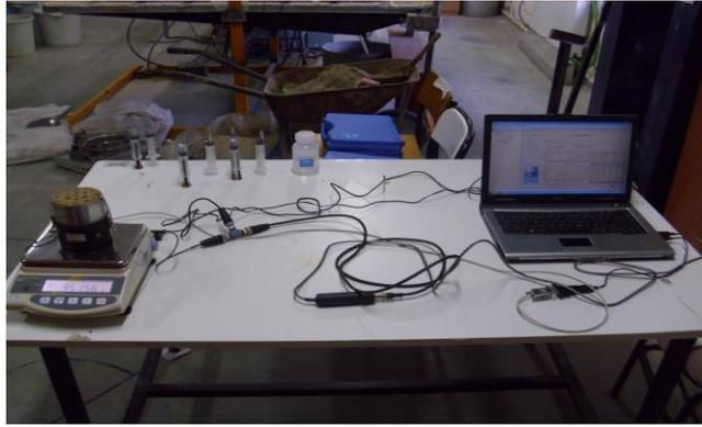
Figure 6.4. Experimental Sets-up of the Hyprop Tests
