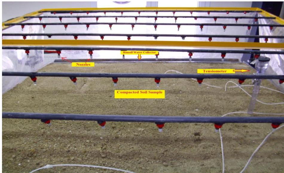
Figure 5.6. Filled Soil Container and Placed-in Tensiometers to Measure Soil-Suction
