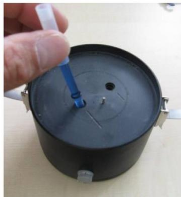
Figure 4.6. Assembly of the Tensiometer
