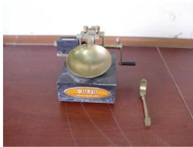
Figure 3.5. Casagrande Apparatus used for the Multi-Point Liquid Limit Test
