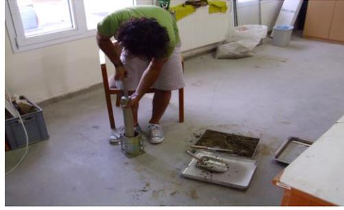
Figure 3.10. Standard Proctor Compaction Test
