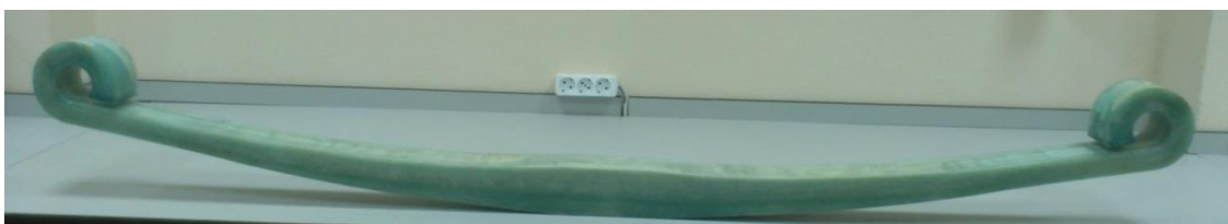
Figure 3.10. Photo of manufactured composite leaf spring based on Design B.
