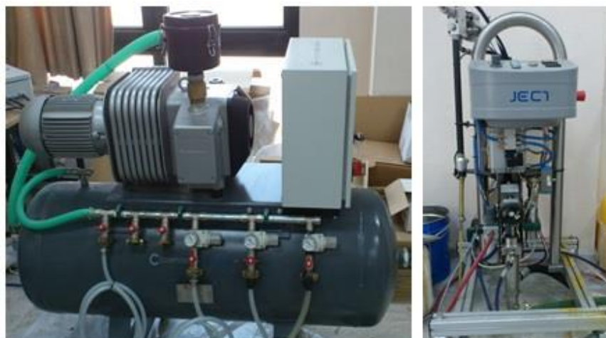
Figure 3 3. Vacuum pump and RTM machine used in the manufacturing stages
