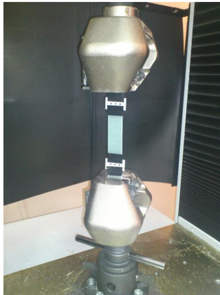
Figure 3.12. Tensile test configuration
