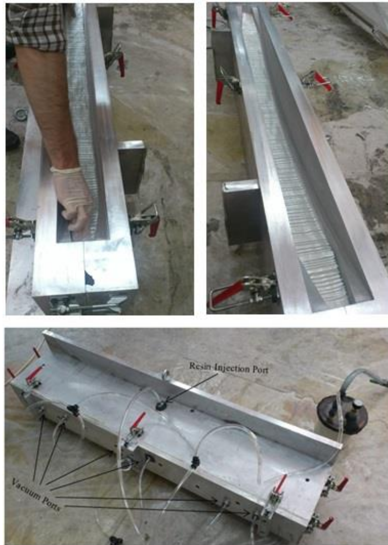
Figure 3.6. Photos showing the RTM stages to manufacture composite leaf spring for Design A
